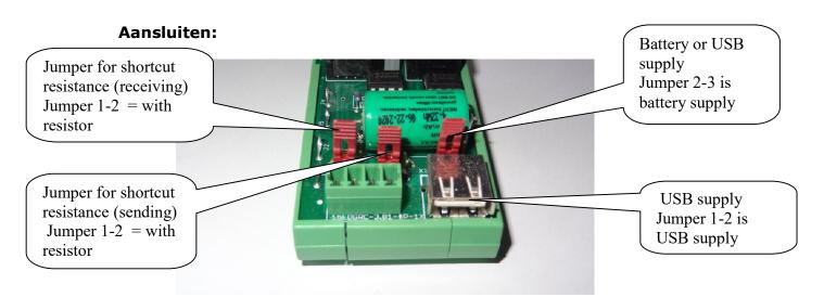
Via RJ45 (sending = pin 1-2) & (receiving = pin 7-8) specially for Master/ Slave/ SL-Server data transfer
